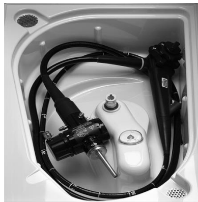
Figure 5: Top view of an automated endoscopic reprocessor (AER) that is used to clean and disinfect the scopes between each use.
